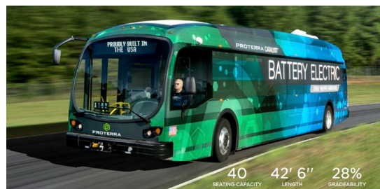
The Proterra Catalyst boasts a range of up to 390 miles and battery capacity of 660kWh
