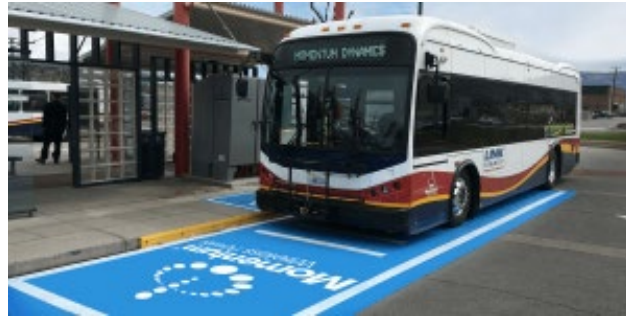
Momentum Dynamics Inductive Charging. Source: electricdrive.com
